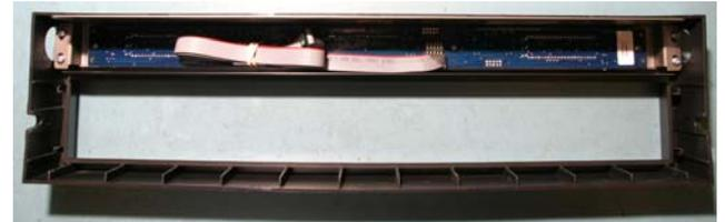
**Figure 1:** Two screws in each side of the display assembly secure it to the bezel. A terminated ribbon cable attaches to the back of the board on the display assembly. A bare ribbon on the front of the board attaches it to the display assembly.
