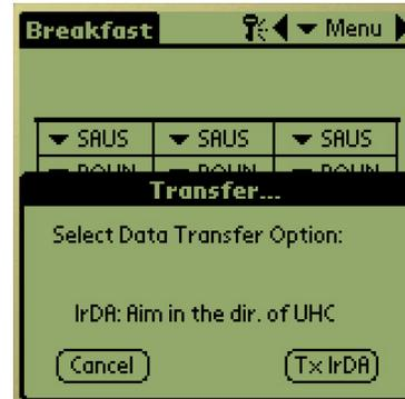
**Step 16:** Ensure the dark receiving lens on the front of the cabinet is clean. Hold the Palm Pilot parallel with the floor and aim it at the lens from no more than one foot away.
